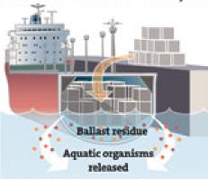
A ship at a foreign port loads cargo and diecharges ballast water. Small marine organisms may be in the tanks' residual water and mud. The ship departs for the Great Lakes.
