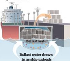
At a Great Lakes port, the ship takes on ballast water as it unloads cargo. The freshwater mixes with the residual water and mud that may contain organisms from a foreign port.
