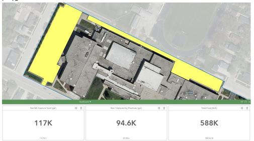
5. Permeable pavement is a powerful tool for turning previously impermeable surfaces into permeable ones. However, it is not without its downsides, such as rougher rides for vehicles and an increased maintenance cost (predominantly from regularly cleaning the gaps between pavers). For these reasons, it may be advantageous to design a scenario using multiple different practices.
