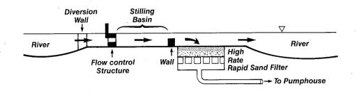
However, sand filter intakes can clog, reducing infiltration rates — a potential problem that can be reduced by oversizing the infiltration area, by careful siting or by providing a back-up storage reservoir.
