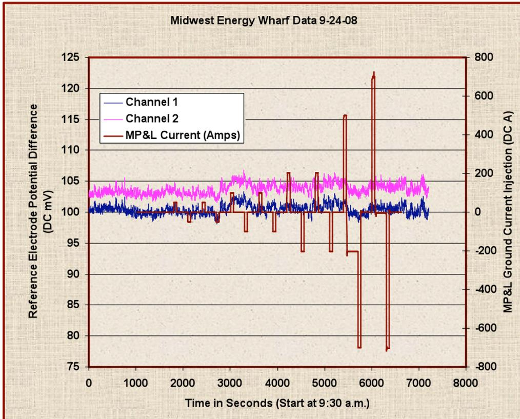
Figure 3b. Field gradient (mV, left) and HVDC ramps (A, right) vs. time at Midwest Energy Wharf
