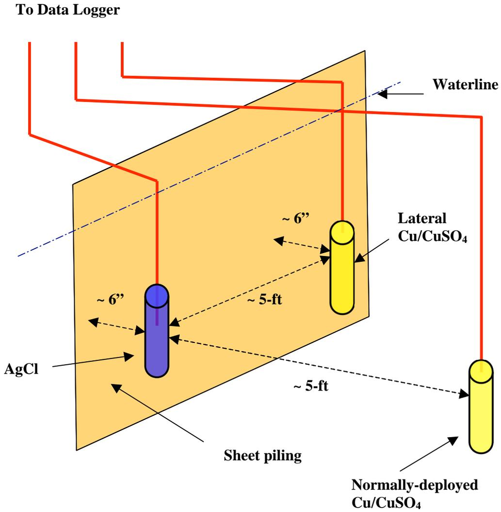
Figure 1. Schematic arrangement of 3 reference electrodes for field-gradient DC potential measurements
