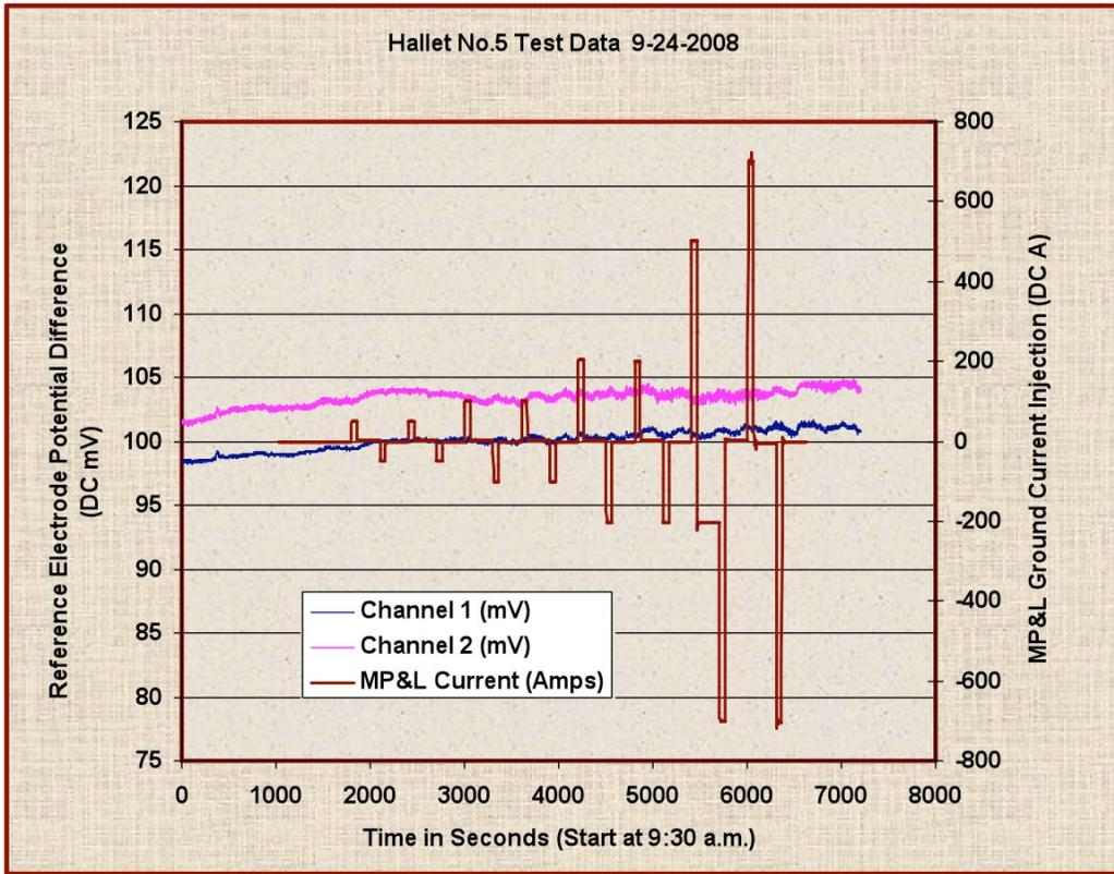
Figure 3a. Field gradient (mV, left) and HVDC ramps (A, right) vs. time at Hallet No. 5
