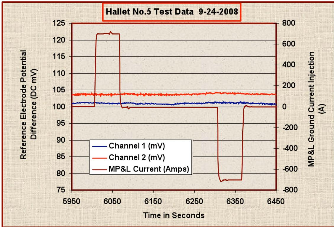
Figure 4a. Field gradient (mV, left) and  $\pm 700\text{A}$  HVDC ramps vs. time at Hallet No. 5 location
