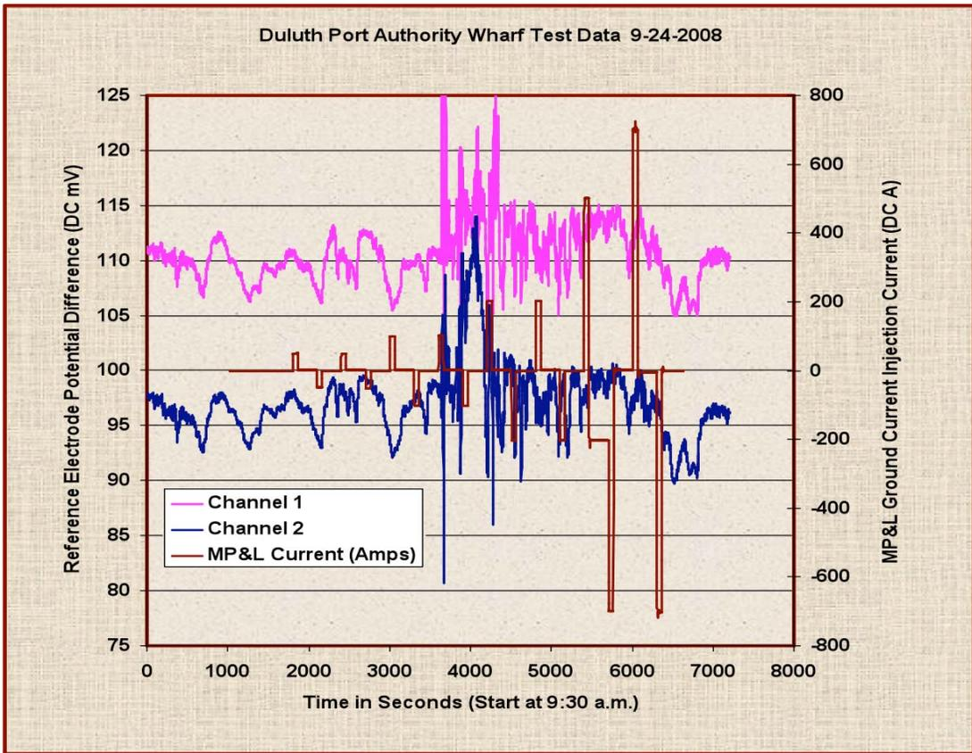
Figure 3c. Field gradient (mV, left) and HVDC ramps (A, right) vs. time at Port Authority
