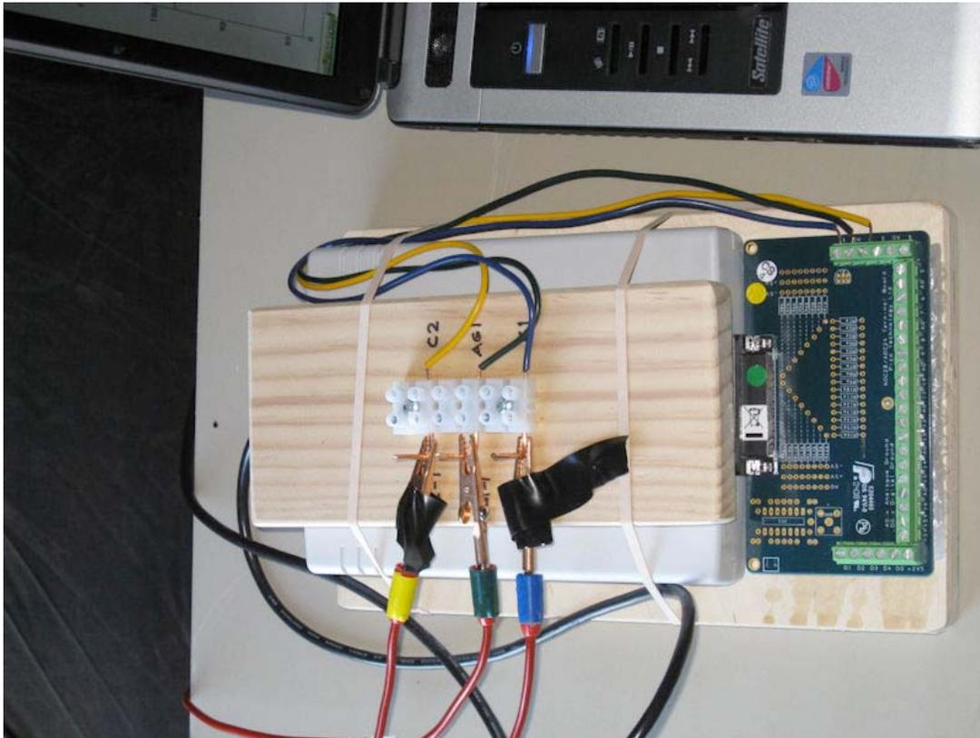
**Custom Terminal Board Showing Connections to Data Logger and Reference Electrodes**
