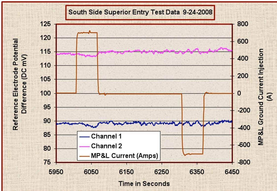
Figure 4d. Field gradient (mV, left) and  $\pm 700\text{A}$  HVDC ramps vs. time at South side Superior entry location
