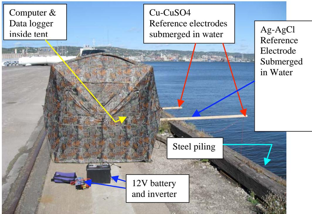
Figure 2a. Typical stray-current field test setup at each location
