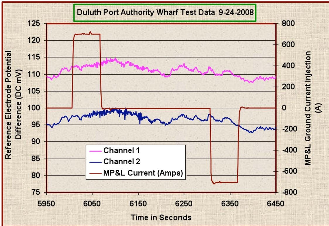
Figure 4c. Field gradient (mV, left) and  $\pm 700\text{A}$  HVDC ramps vs. time at Port Authority Wharf location
