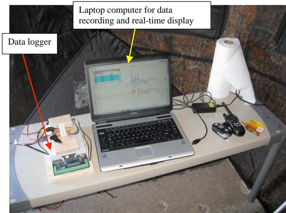
Figure 2b. Typical data logging system setup
