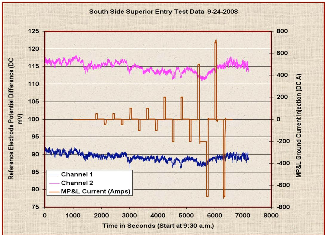
Figure 3d. Field gradient (mV, left) and HVDC ramps (A, right) vs. time at South Side Superior entry
