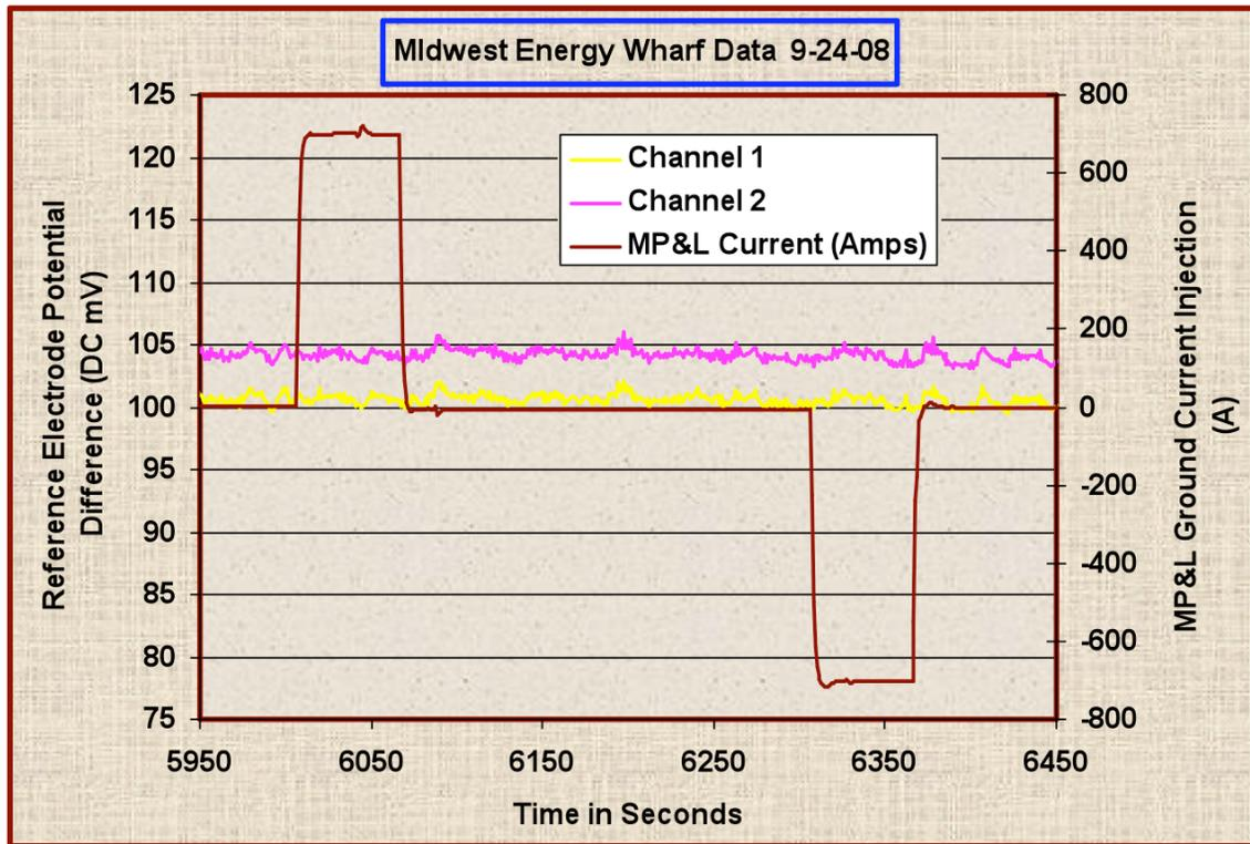
Figure 4b. Field gradient (mV, left) and  $\pm 700\text{A}$  HVDC ramps vs. time at Midwest Energy Wharf location
