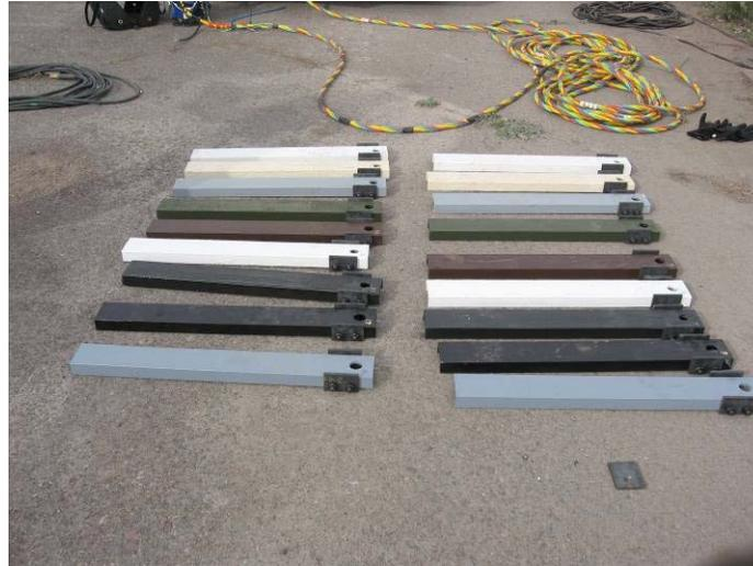
**Picture 1: Uninstalled Ice Abrasion Samples**
