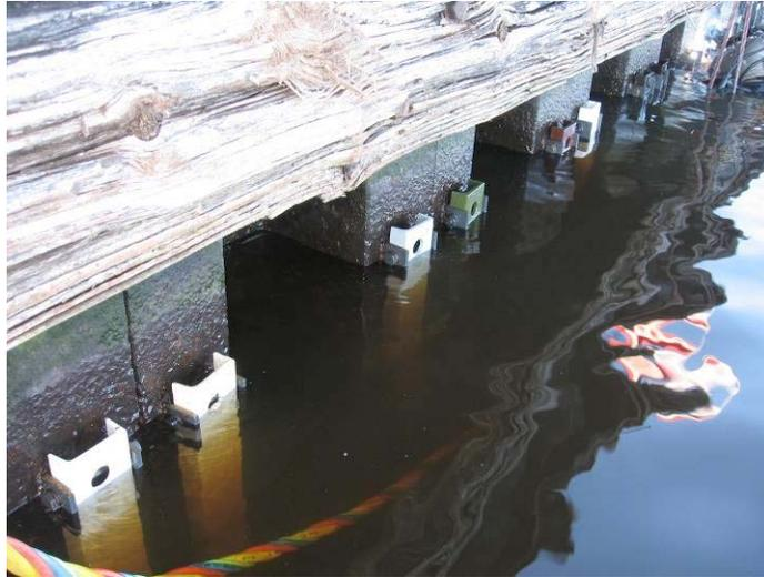
**Picture 2: Installed Ice Abrasion Samples**
