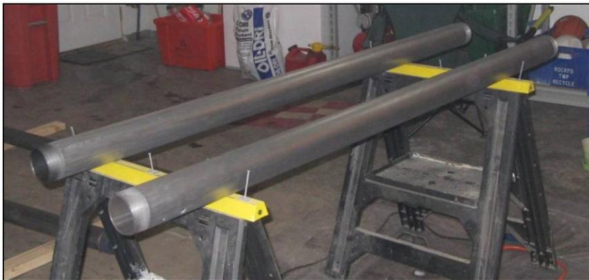
Pipes were sandblasted and cleaned before any coating was applied.
