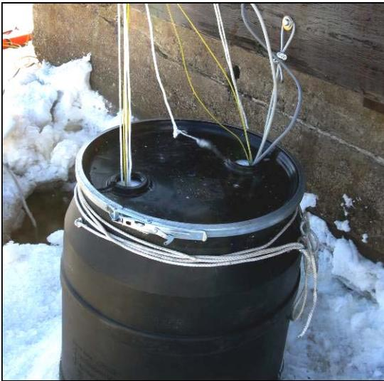
Each barrel cover was insulated for further freeze protection. The covers can be removed to allow pipes & anodes to be removed and inspected during winter months as well as allowing water conductivity measurements.
