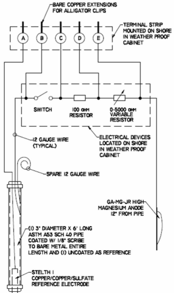
**Figure 5: Testing Procedures & Electrical Schematic**
