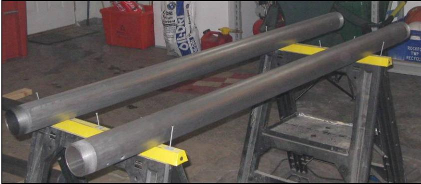
Test samples shown after sandblasting and prior to installation of coating, wires, and hardware.
