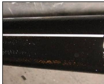
After coating the tape was removed and a 1/8” scribe line results the length of the pipe.
