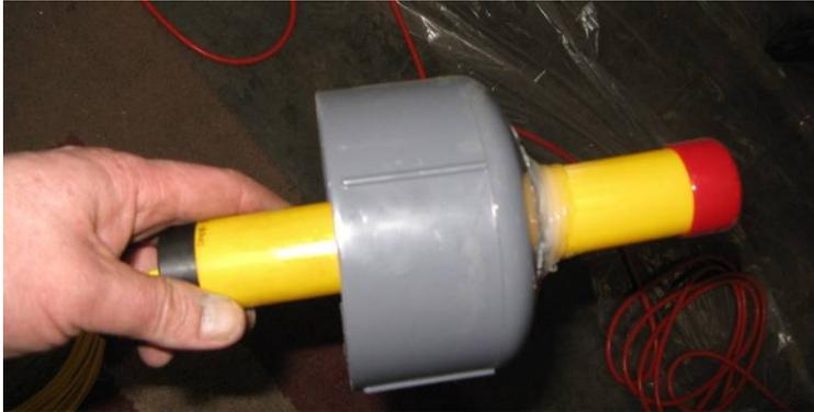
The reference electrodes (shown with protective red cap) were inserted through holes in the bottom pipe caps of samples, glued to caps, and sealed.
