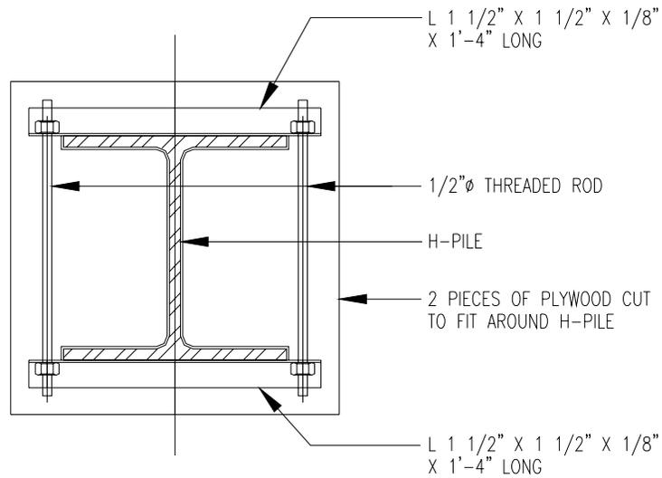
**Figure 3: Series 500 H-Jacket Base Plate Detail**
