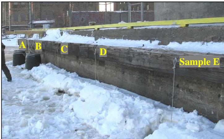
Samples were installed 10 feet apart from each other along pier to avoid any electrical interference between individual pipes. All except C were isolated from existing steel structures.
