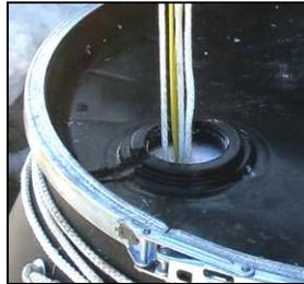
Slots were cut to allow the wires, cables, and rope to pass through and covers to be removed.
