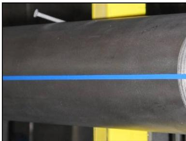
A 1/8” wide vinyl tape was applied the length of pipe prior to coating.
