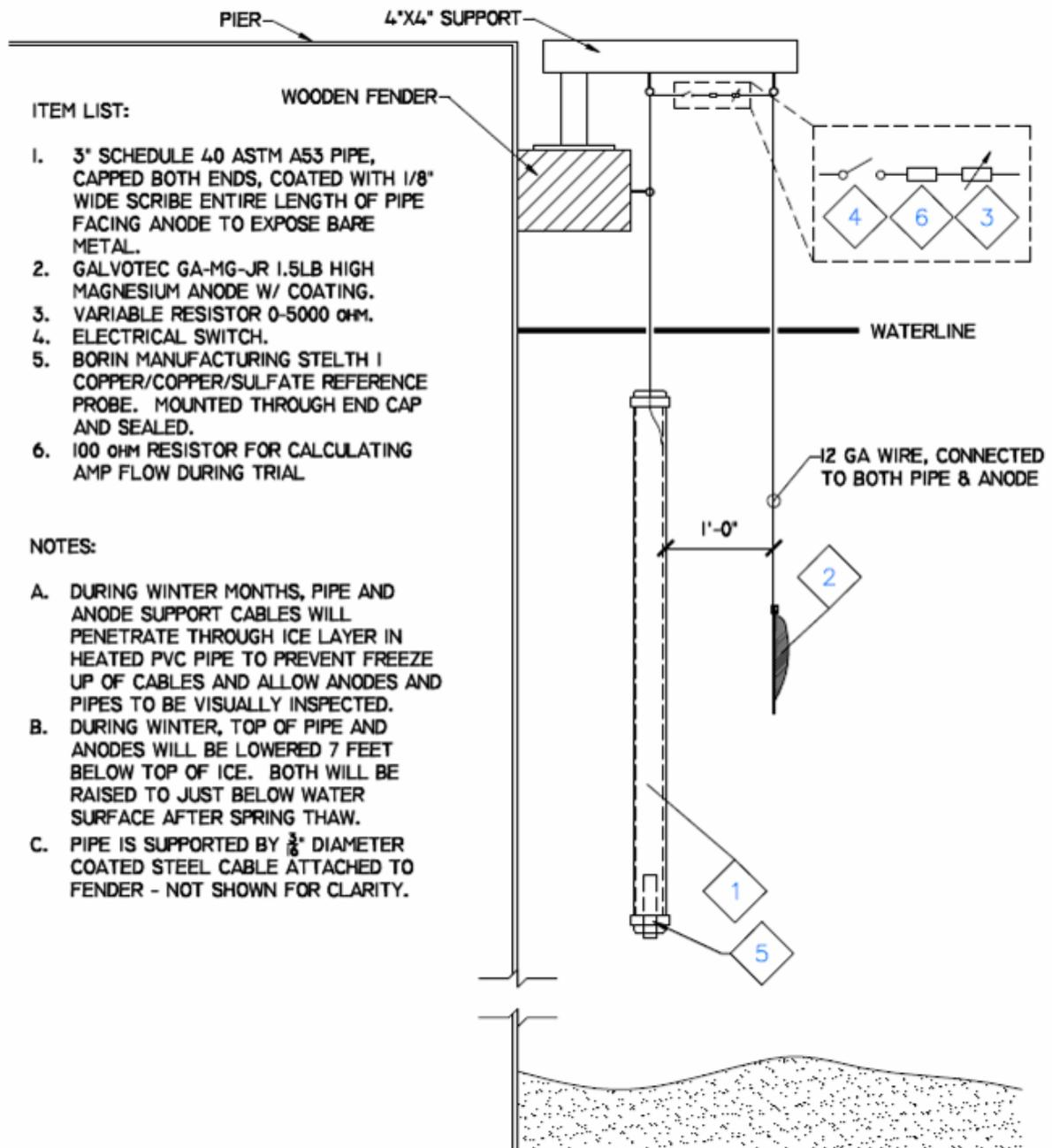
**Figure 4 – Sample A Installation Schematic**
