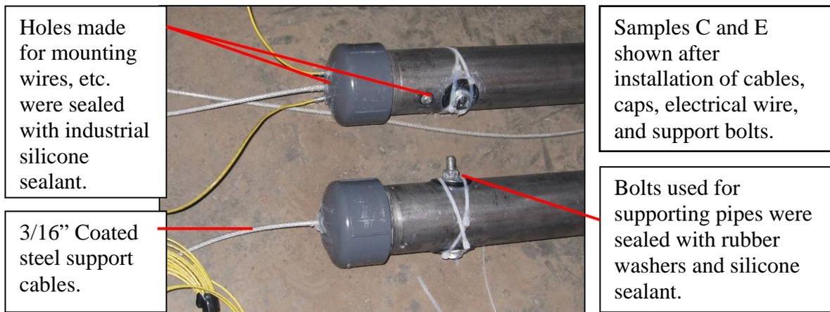
**Picture 20: Pipe Sample Sealing**
