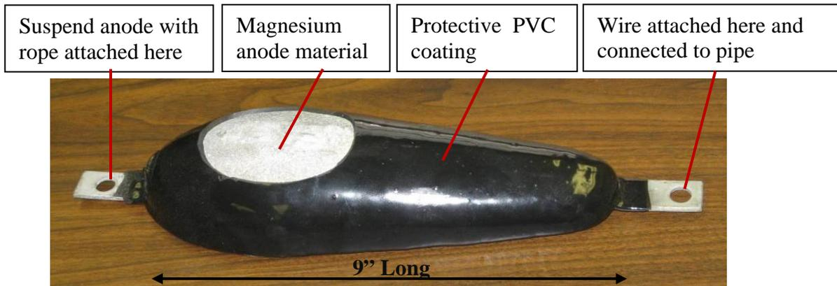
**Picture 13: High Magnesium Anode Used for Trial**
