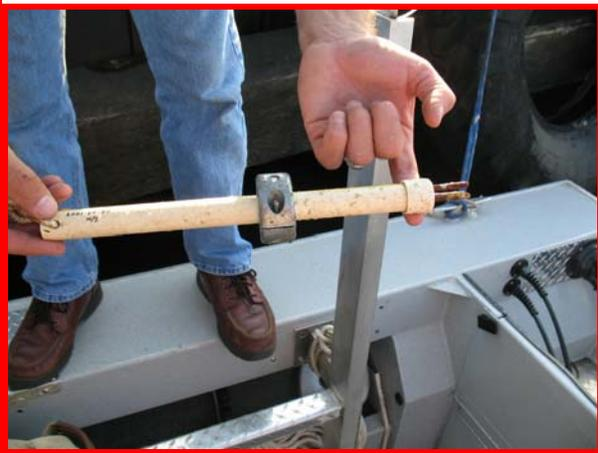
Figure 3 - LPR Probe after 1 week exposure
