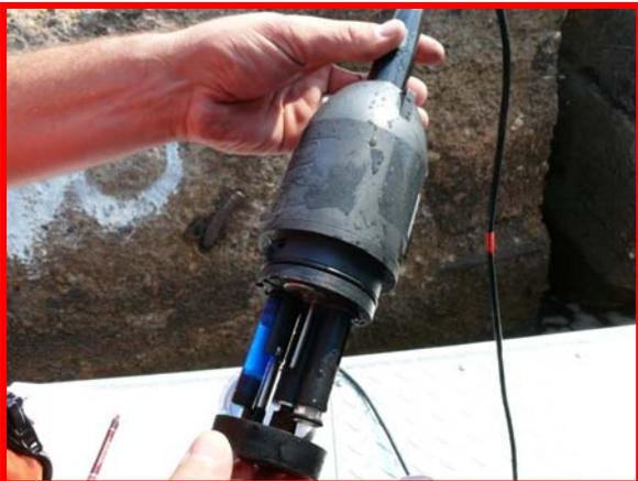
Fig 10 – AMI Hach Water Chemistry Probe
