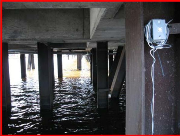
Figure 2 - LPR Test Probe Junction Box
