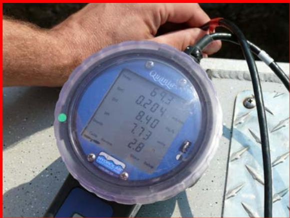
Fig 11 – Hach Water Chemistry Display
