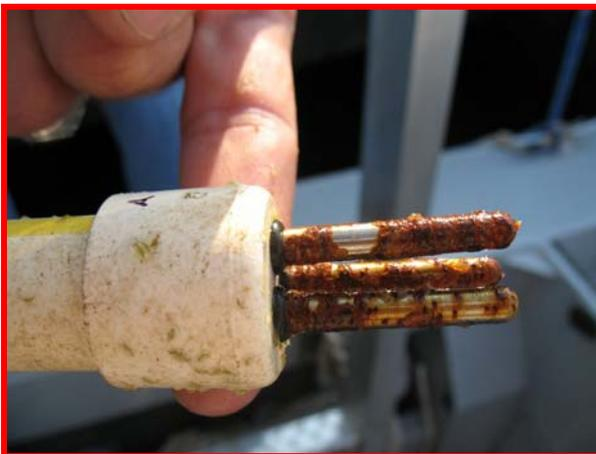
Figure 4 - LPR Test Probe Tips after 2 weeks exposure
