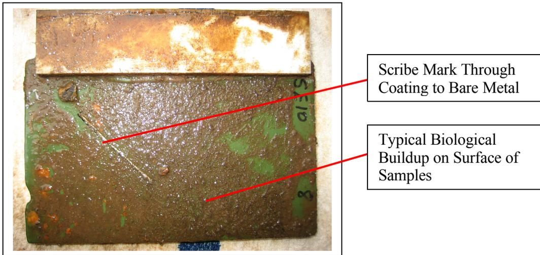
**Figure 3. Coated Test Coupon**
