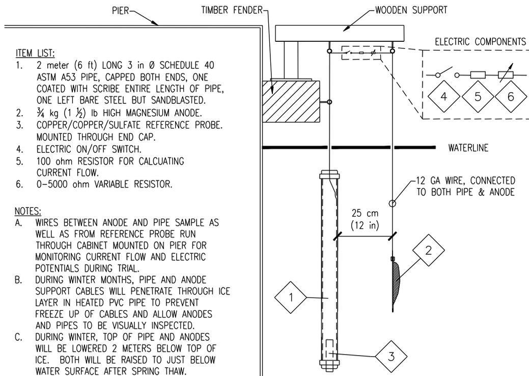
**Figure 5. Cathodic Protection Test Schematic**
