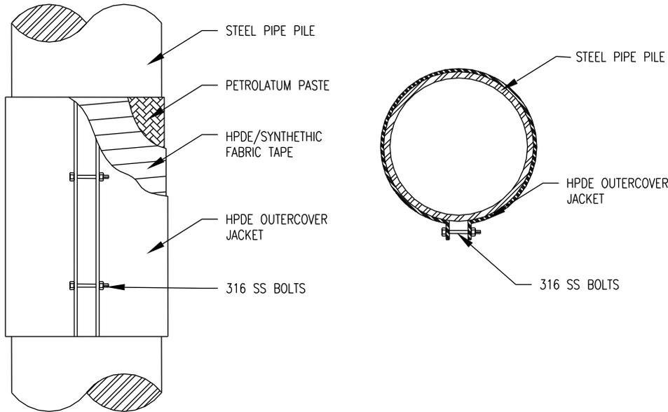
**Figure 7. HPDE Pipe Pile Protective System**
