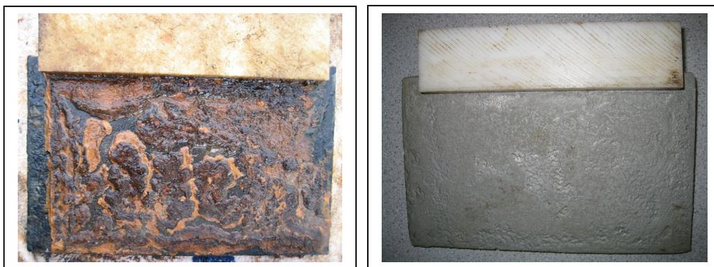
**Figure 2. Uncoated Test Coupon Before and After Cleaning**
