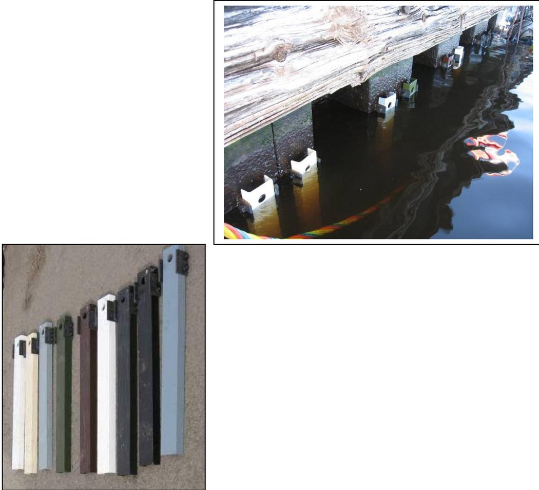
**Figure 4. Ice Abrasion Samples Before and After Installation**
