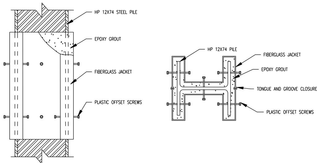
**Figure 6. H-Shaped Fiberglass Protective System**
